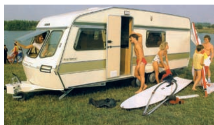
GRP front panels on Clubman and Delta ranges make the profile more aerodynamic to improve towing and the van's look
