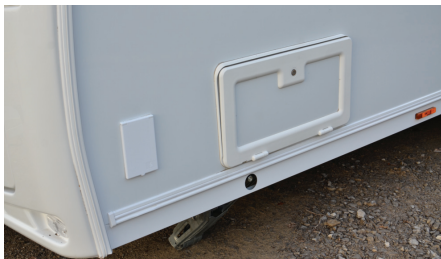
Barbecue point and external side locker, along with heavy duty corner steadies.
